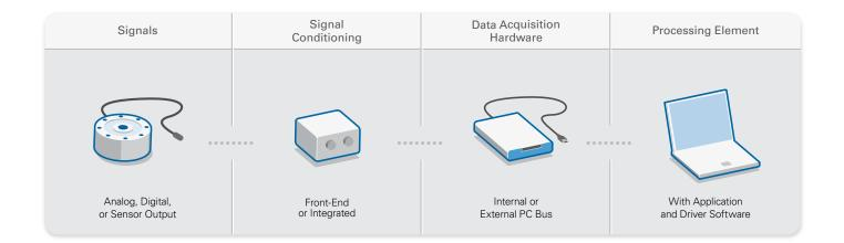
You can use data acquisition tools for a variety of applications such as data logging, control, and test automation on any bus with easy, powerful software.
