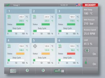
additional indicating instruments are no longer required. An extensive alarm system, the trend graphs, and loading and storage of production data increase process safety and product quality.
