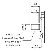
Shaft Detail - SAE "CC" Spline
