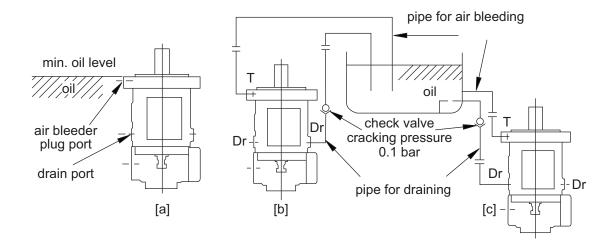
A check valve with cracking pressure of 0.1 bar should be fitted to the case drain line as shown. Recommended Kawasaki check valves are as follows: (refer to Kawasaki industrial valve information - data sheet C1001)
