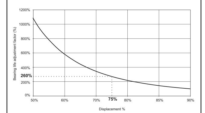
All bearing life curves on the previous pages refer to L10 life at full displacement. The foregoing curve is therefore to be used where duty cycle considerations require one to compute weighted life, which include partial displacement conditions.
